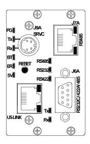
Remote control link ..... US-LINK (RJ-45) BITE .....Included Weight .....8oz Operating temp .....0 to +70C Non-operating temp ....-20 to +85C Humidity .....0 to 95% (NC @ +25C) MTBF .....>225,000 hours (per MIL-HDBK-217F, N1 ground benign @ +25C)
